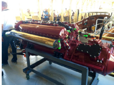
One of two Allison V-12 aircraft engines used to power the Thunderbird yacht.
