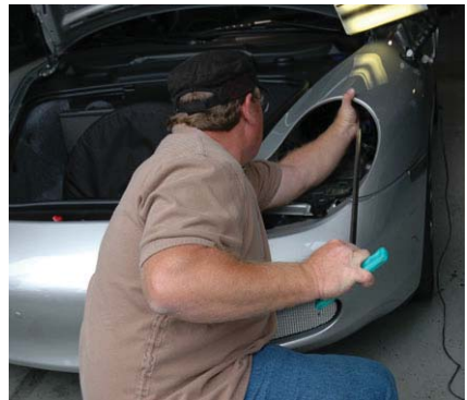
Joe removed the headlight from this Boxster to provide access for one of the many tools used to ease out the little dents that are his bread and butter.
