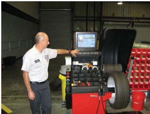
Dave demonstrates tire balancing and road force measurements.
