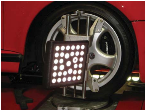
Alignment tool with 33 circles mounted on the right front wheel.
